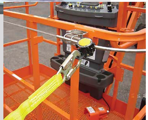
Photos 3 and 4 (above, right): The pictured aircraft external fall arrest anchorage subsystem allows one worker limited excursions outside of the MEWP, if the jobsite and local restrictions allow. Specific guidelines for use and inspections are in the operator's manual and must be followed.
