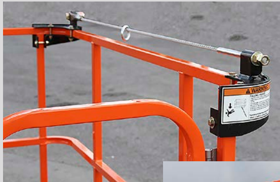
Photo 1 (above): An anchorage subsystem that allows for limited excursions outside of the MEWP, if jobsite or local restrictions allow.
