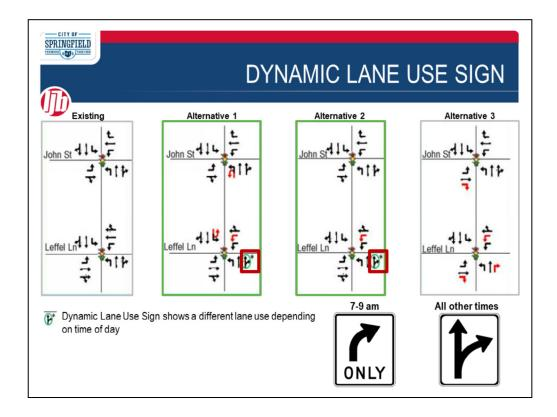
Alternatives 1 and 2 would utilize a Dynamic Lane Use sign, which uses LED lights to show a different lane use sign depending on the time of day. Between 7 am and 9 am, the right northbound lane at Leffel Lane would permit right turns to eastbound Leffel Lane only. At any other time of day, this lane would permit both through movements and right turns.
